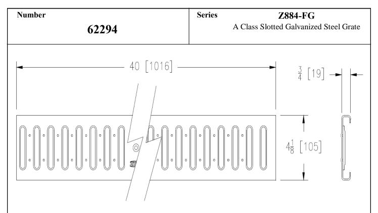
The Zurn Z884-FG Fabricated Galvanized Slotted Grate is 4-1/8+wide x 40+long weighing 1.8 lbs. per linear foot. The grate has an open area of 10.2 square inches per linear foot, DIN rating of Class A, ANSI rating Light-Duty. Supplied by Trench Drain Supply.
