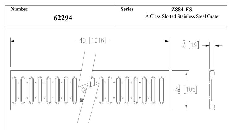
The Zurn Z884-FS Fabricated Stainless Steel Slotted Grate is 4-1/8+wide x 40+long weighing 1.8 lbs. per linear foot. The grate has an open area of 10.2 square inches per linear foot, DIN rating of Class A, ANSI rating Light-Duty. Supplied by Trench Drain Supply.
