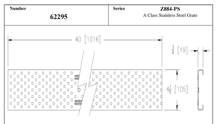
The Zurn Z884-PS Stainless Steel Perforated Grate is 4-1/8+wide x 40+long weighing 1.2 lbs. per linear foot. The grate has an open area of 5.9 square inches per linear foot, DIN rating of Class A, ANSI rating Light-Duty, ADA compliant. Supplied by Trench Drain Supply.
