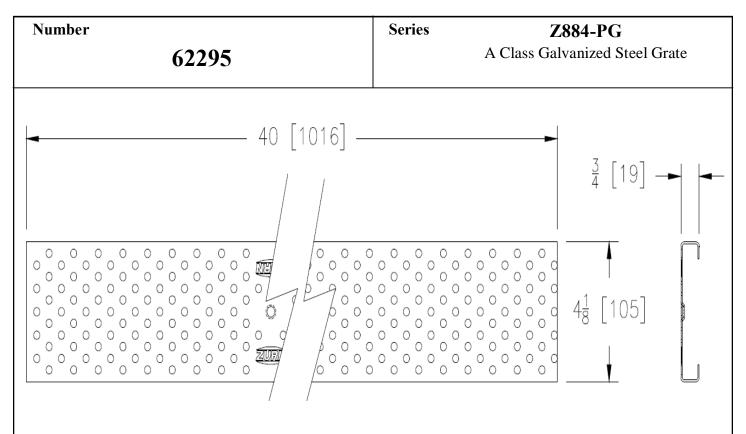
The Zurn Z884-PG Galvanized Steel Perforated Grate is 4-1/8+wide x 40+long weighing 1.2 lbs. per linear foot. The grate has an open area of 5.9 square inches per linear foot, DIN rating of Class A, ANSI rating Light-Duty, ADA compliant. Supplied by Trench Drain Supply.
